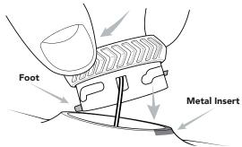
**b.** Press the reel firmly into the collar (you should hear a "CLICK" when secure).
