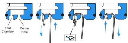
\*\*MAKE SURE THE KNOT DOES NOT INTERFERE WITH THE CONNECTION OF THE SNAP\*\*
