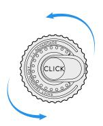
To fully release lace, unwind counterclockwise until "clicking" stops. Lace will then freely release from the reel.
