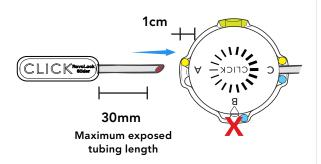
**d.** Place Lamination Collar and Slider Base in desired location.
