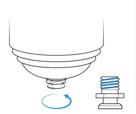
21) Test the snap connection by attaching and detaching 2-3 times.
