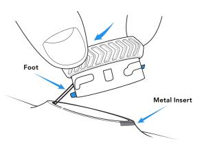
**b.** Press the reel firmly into the collar (you should hear a "CLICK" when secure).
